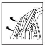
Gently pull the radiator cover/front grill toward you and pull the front grill trim bar away from the headlamp lens. The front grill bar is attached to the headlamp lens with a hidden clip.
